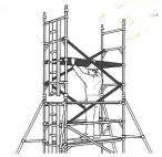
5 Climb the ladder and from the protected position of the trapdoor, fit guardrails to the 7<sup>th</sup> and 8<sup>th</sup> rungs (in that order), on both sides of the tower.
