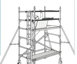
6 Fit the next pair of diagonal braces in opposing directions between the 3<sup>rd</sup> and 5<sup>th</sup> rungs. Add 2 additional end frames.
