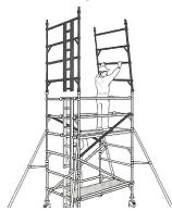
7 If finishing at this height, (4.2m platform), the fixed deck should first be repositioned to the 8\* rung of the tower. Fit a trapdoor deck alongside it, with the trapdoor next to the ladder.
