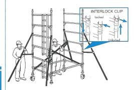
5 Fit a fixed deck on lowest rung. Fit a trapdoor deck on 4th rung (2.0m) with the trapdoor next to the ladder. Climb ladder and, from a protected trapdoor position, fit guardrails on 5<sup>th</sup> and 6<sup>th</sup> rungs, in that order, on both sides of the platform.
